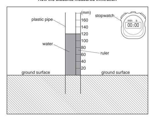
The students used a **plastic pipe** which they pushed into the ground to the same depth at each site. The students put a **ruler** which measured in millimetres inside the pipe. They poured water into the pipe up to a height of 120 mm. They recorded the water height in the pipe after 10 minutes, timed by a **stopwatch**.
